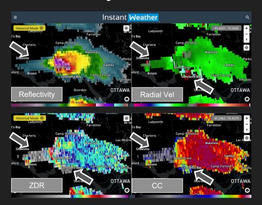
ZDR: the difference between the horizontal and vertical returned power - shape *CC*: a measure of the consistency of the shapes and sizes of targets - similarity
